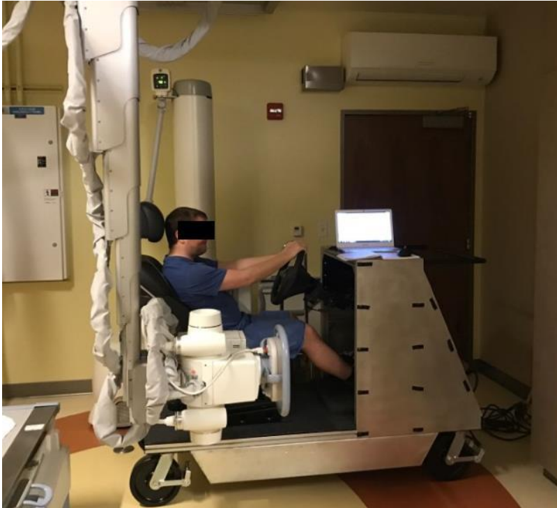
Fig1. The mock-up carseat with a steering wheel is set up in the x-ray room for lateral x-ray acquisition.
