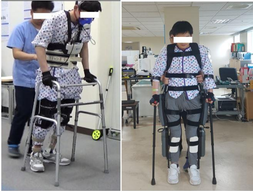
Fig 1. The patient walking over ground with KAFO and ReWalk™ for gait training
