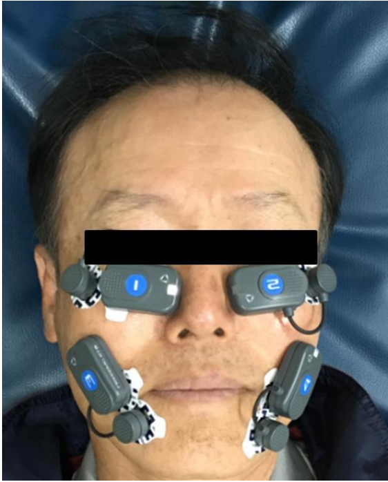
Fig 1. Recording sites of surface electromyography (BTS FREEMG 1000, BTS Bioengineering, Milano, Italy). Four electrodes were attached bilaterally over bilateral orbicularis oculi and orbicularis oris muscles.
