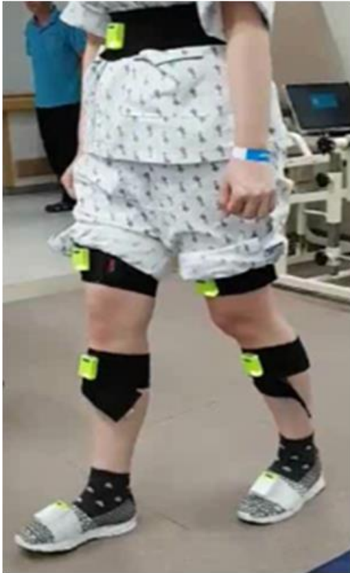
The 3-dimensional gait analysis system with IMU sensors
