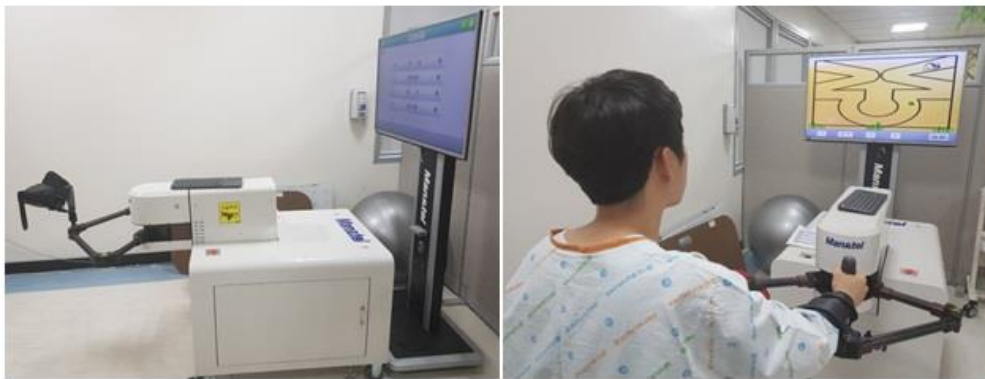
Figure 1. (A) Camillo® robotic device, an upper extremity rehabilitation robot, consisting of a video monitor, a robot arm and a computer: (B) The patient performing robot-assisted game training with the upper extremity rehabilitation robot.
