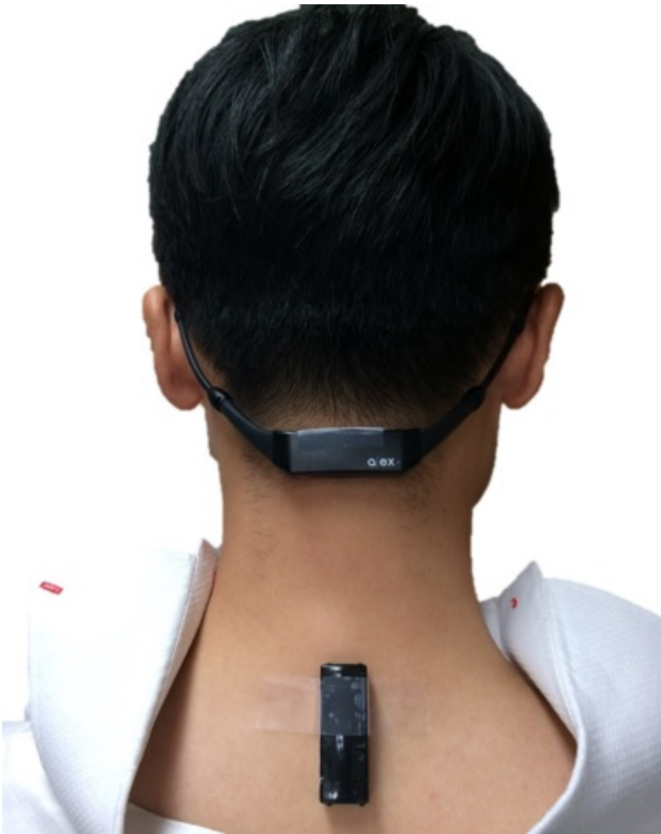
Fig. 1. Two wearable sensors to measure neck and back flexion angles.
